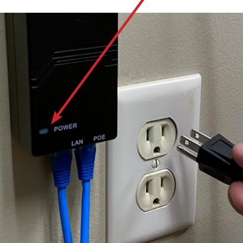
2. Reconnect POE connection ensuring that the power indicator is illuminated. Allow the system to complete the booting process for a period of 5 minutes.
