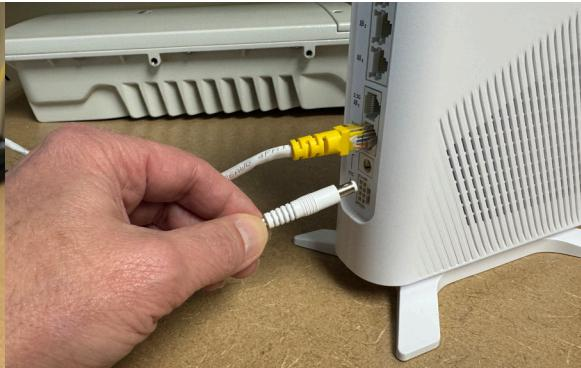
**5.** Connect the router and wait for a 5 minute period before proceeding to test the Internet service.
