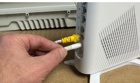
**4.** Locate the router and disconnect the power supply. Wait for 10 seconds.
